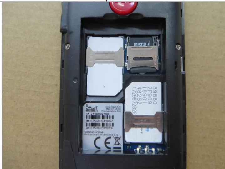
SIM card and TF installation check
