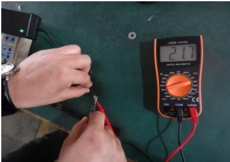
Charger output voltage check
