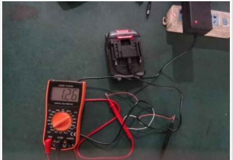
Charger output current check
