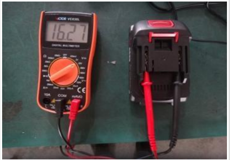
Battery voltage after discharge
