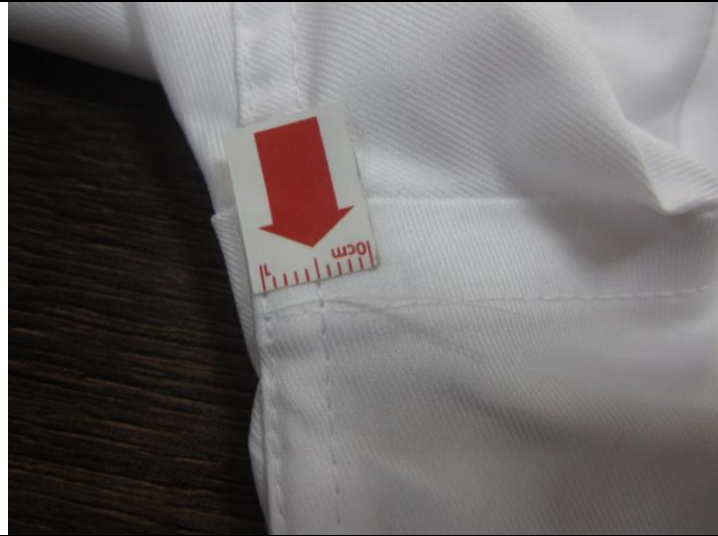
Untrimmed thread on armhole-min
