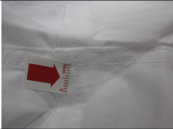
Untrimmed thread on armhole-min
