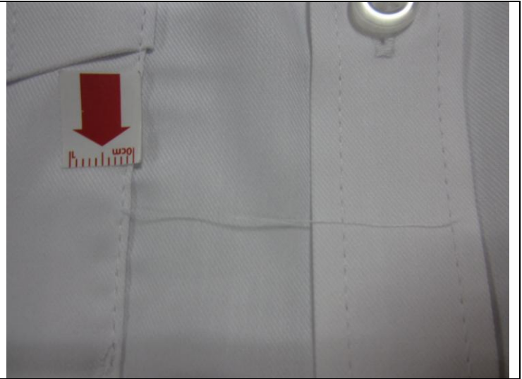
Untrimmed thread on pocket-min
