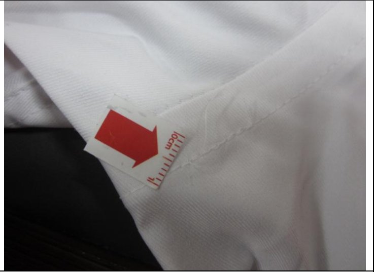
Untrimmed thread on armhole-min
