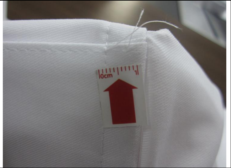
Untrimmed thread on armhole-min
