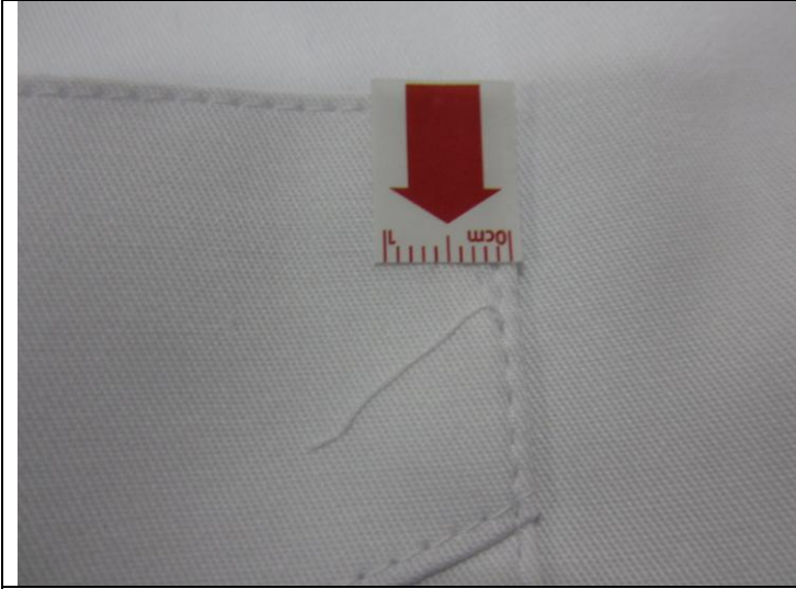
Untrimmed thread on pocket-min
