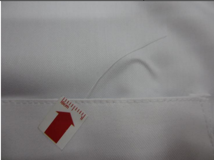
Untrimmed thread on pocket-min
