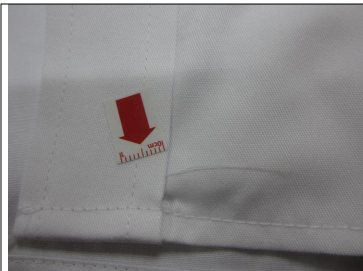
Untrimmed thread on hem-min
