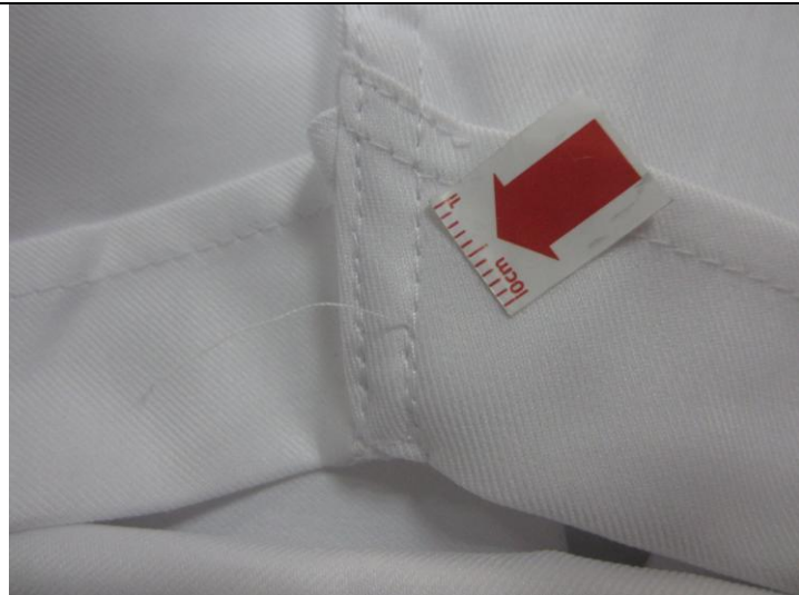
Untrimmed thread on armhole-min
