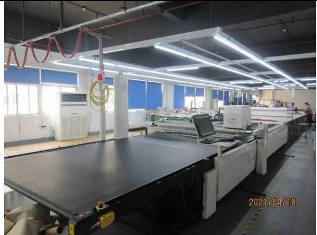
Computerized cutting machine
