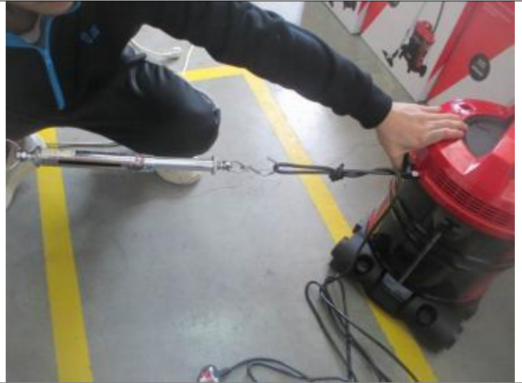
Power cord strain relief test
