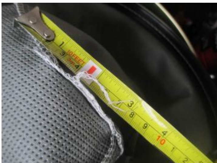
Untrimmed thread end on soft filter bag (4cm) -- Min
