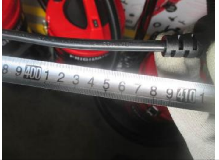
IMG_220 Length of power cord check
