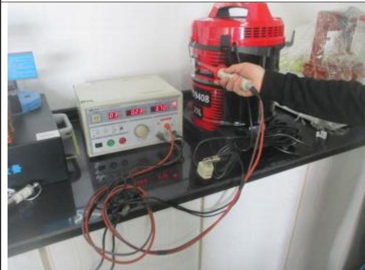
High voltage test
