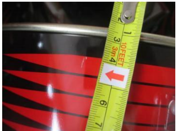
Scratch mark on surface (0.8- 1.5cm) -- Min
