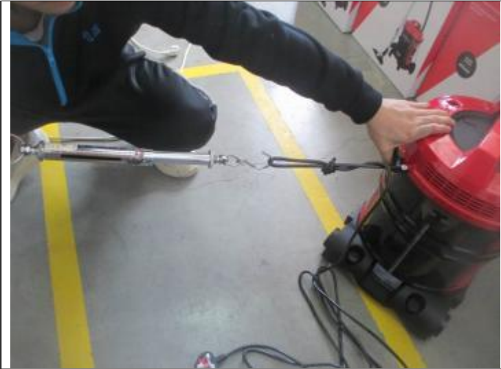
Power cord strain relief test
