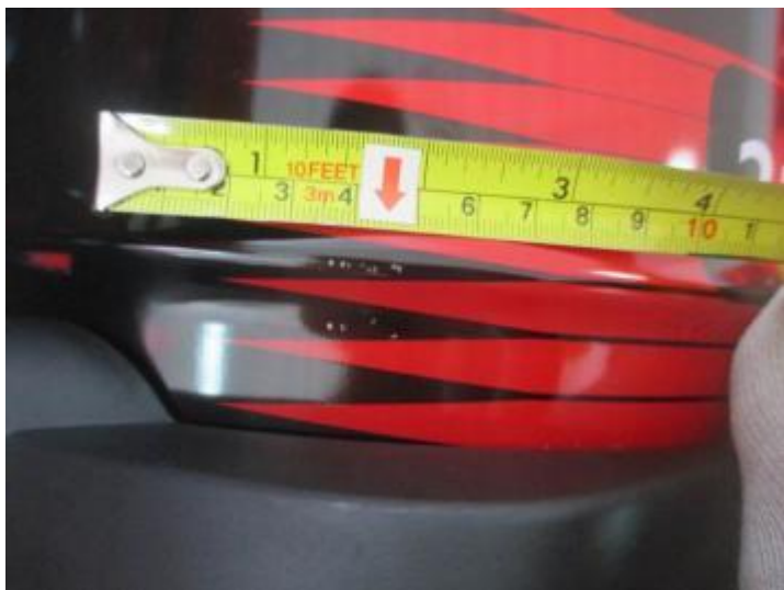
Scratch mark on surface (0.8- 1.5cm) -- Min
